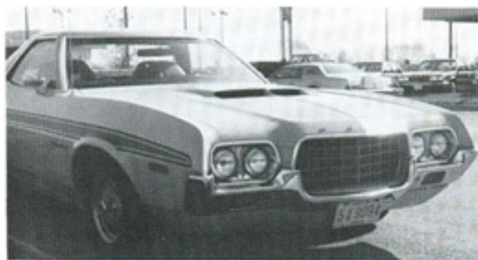
1972 Ranchero GT hood with twin-scoop design. The GT also used a two-tone argent grille. Bumper guards were options. (Bill Holder)
